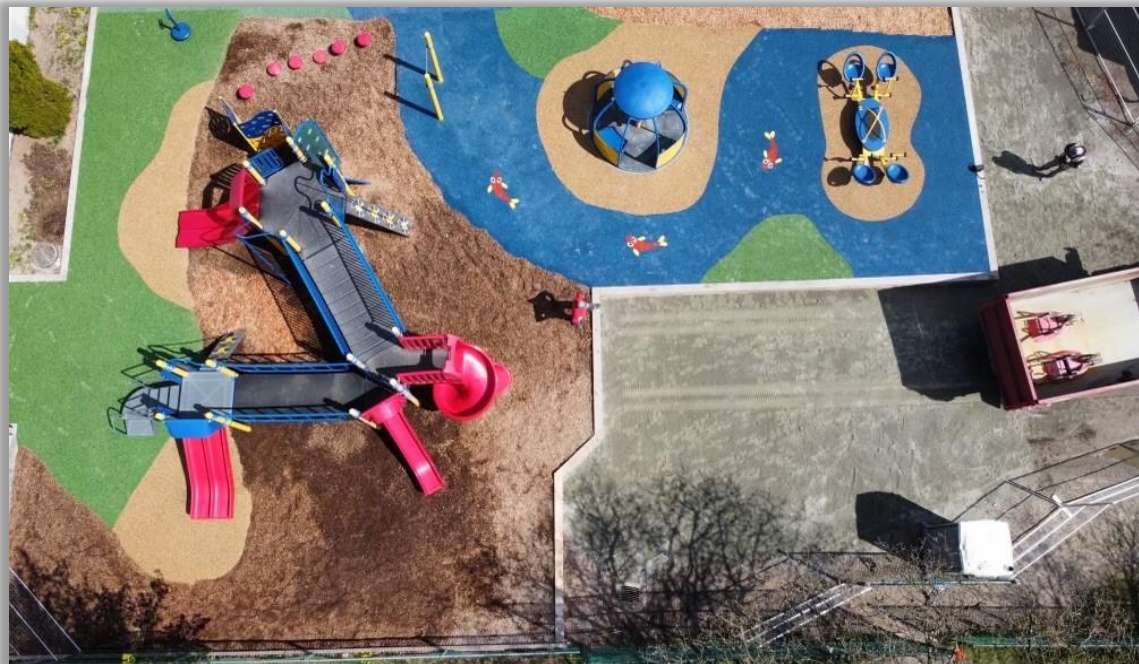
Birdseye view of new playground at McBride Elementary. Note the mix of both poured-in-place rubber and engineered wood fiber surfacing
