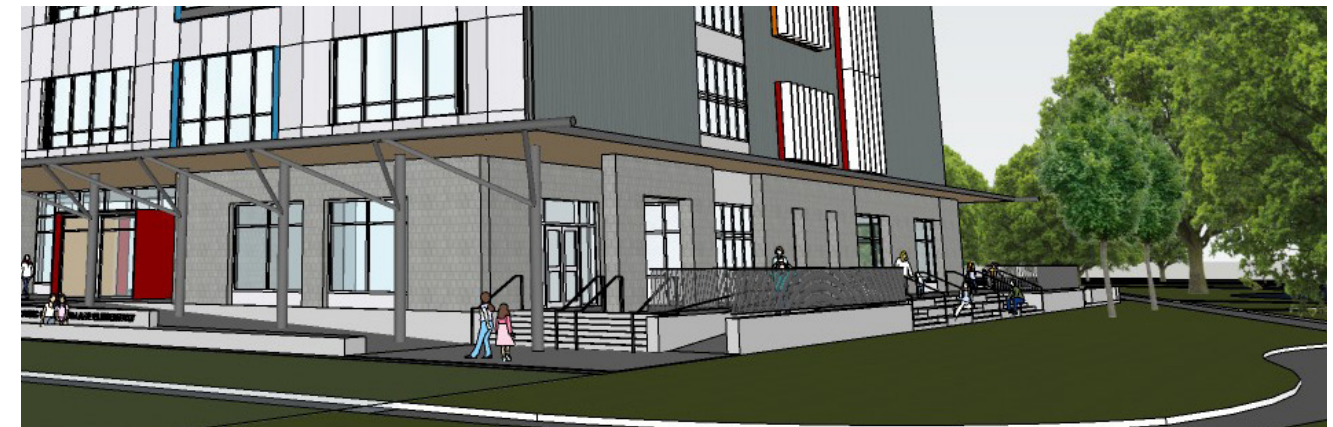
Walkway (sloped at 1:20) leads to main entry and accessible ramp leads to west porch.
