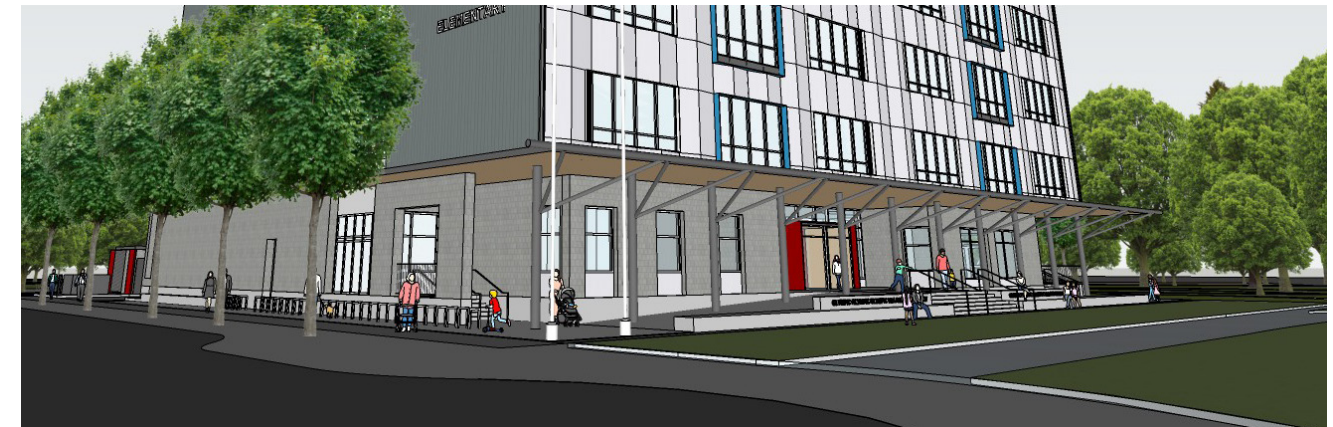
Two walkways (sloped at 1:20) connect the main entry to the sidewalks and north play zone.
