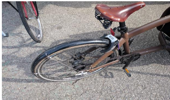
Figure 12: Example of a frame lock on a bicycle.
