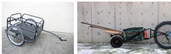
Figure 28: Examples of rear trailers with two wheels (left) and one wheel (right).
